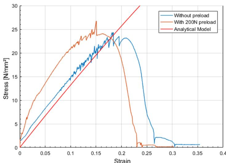
**Figure 4:** Mechanical response of composite bow-tie structure
