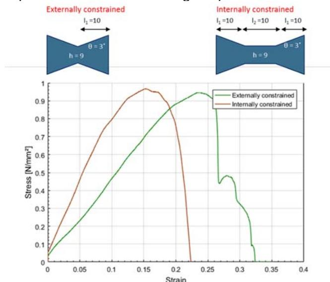
**Figure 3:** Mechanical response of 3D printed bow-tie structures
