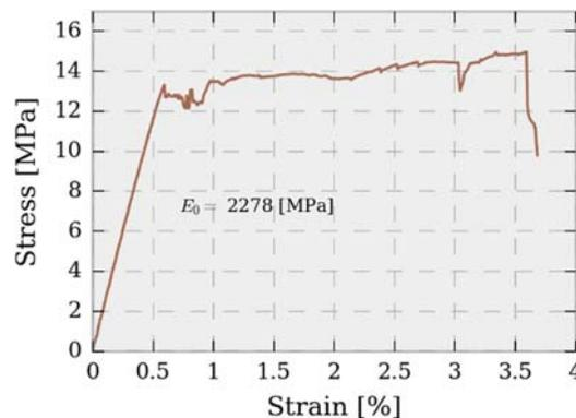
**Figure 2:** Pseudo-ductile behaviour achieved in interlocking ceramic structure
