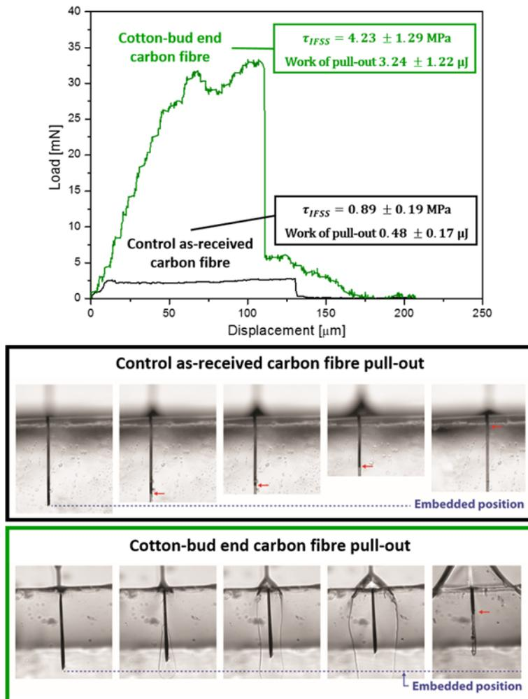
**Figure 2.** Modified single fibre pull-out tests from a compliant matrix.
