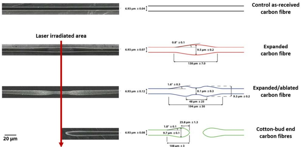
Figure 1. Laser irradiated carbon fibres and the various shapes produced.
