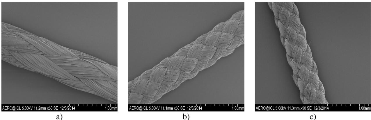
**Figure 1:** Hybrid microbraids: (a) HMB1  $\alpha=14^\circ$  (b) HMB2  $\alpha=33^\circ$ ; (c) HMB3  $\alpha=39^\circ$ .
