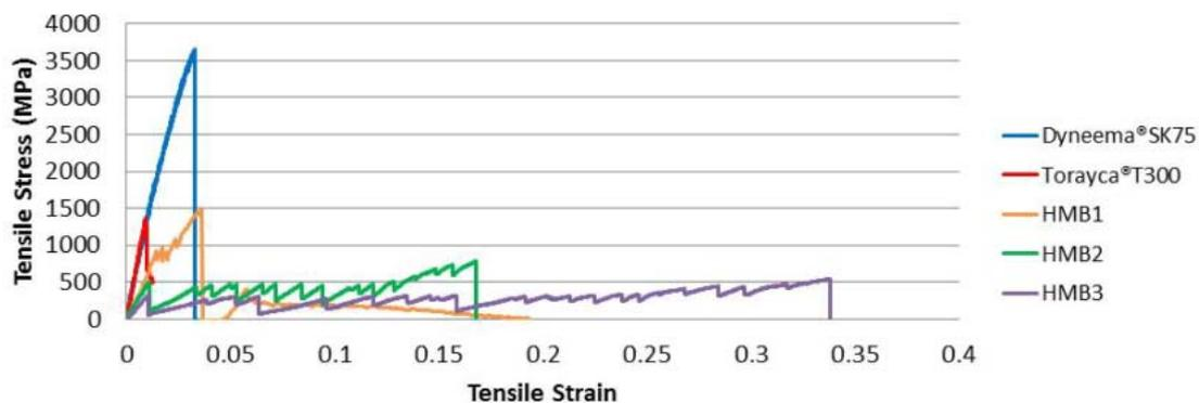
**Figure 2:** Tensile stress vs. tensile strain of the investigated yarns and microbraids.
