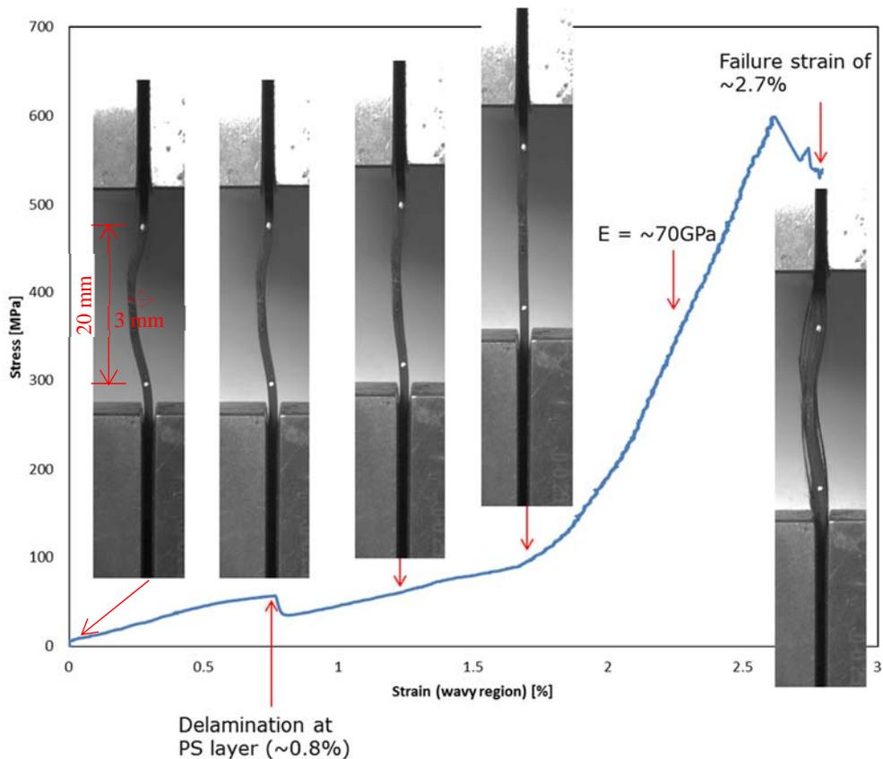
**Figure 2.** Resulting stress-strain relationship of an interleaved wavy specimen under tension at room temperature.
