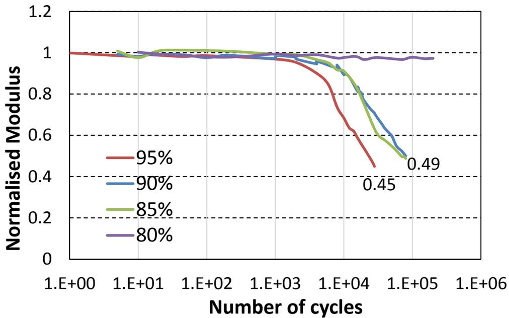
Figure 6. Fatigue response of IM-HM  $[\pm 25_2/0]_s$  laminates
