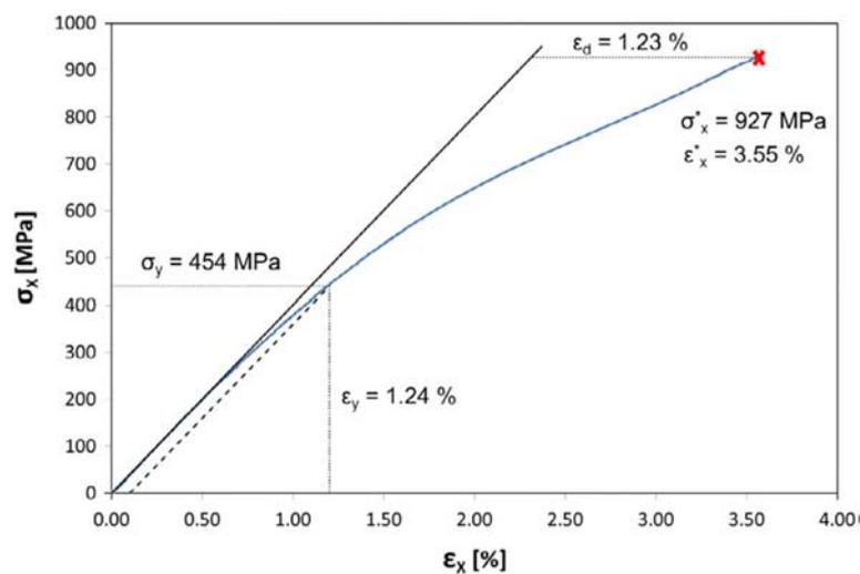
Figure 2. Pseudo-ductile response of thin ply ( $\pm 25$ ) carbon/epoxy laminate
