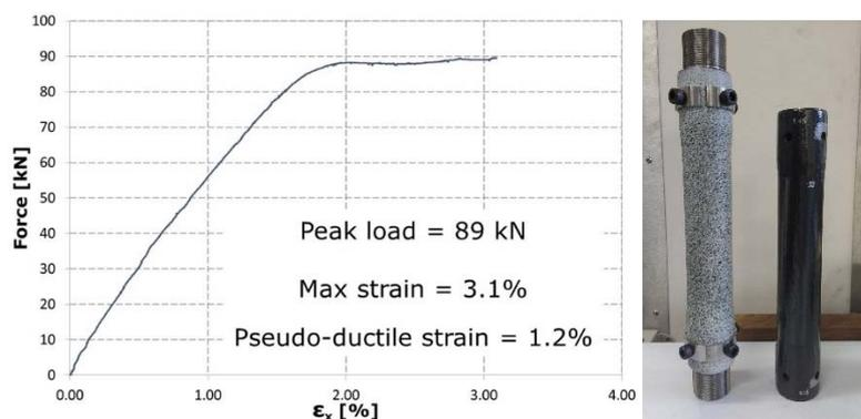
Figure 7. Pseudo-ductile response of tubular tension member
