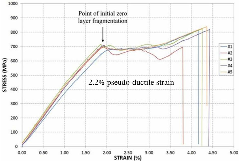
**Figure 4.** Pseudo-ductile response of  $[\pm 26_5/0]_s$  laminate
