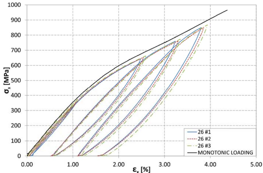
**Figure 3.** Cyclic loading of  $(\pm 26)_s$  carbon/epoxy laminate
