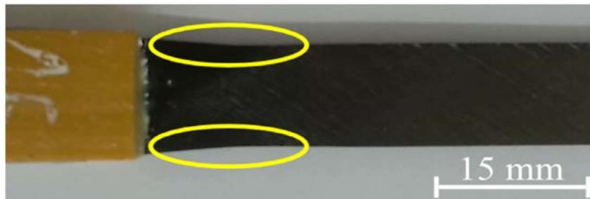
Figure 1. Necking of ( $\pm 45$ ) thin ply carbon/epoxy angle ply specimen
