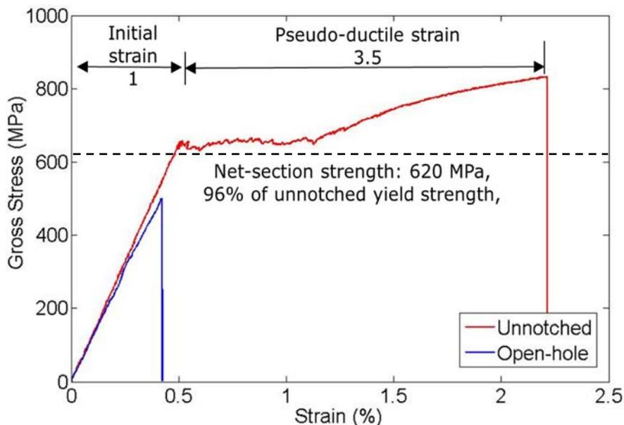
**Figure 5.** Open-hole tension response of  $[\pm 25_2/0]_{s4}$  IM-HM carbon/epoxy laminates
