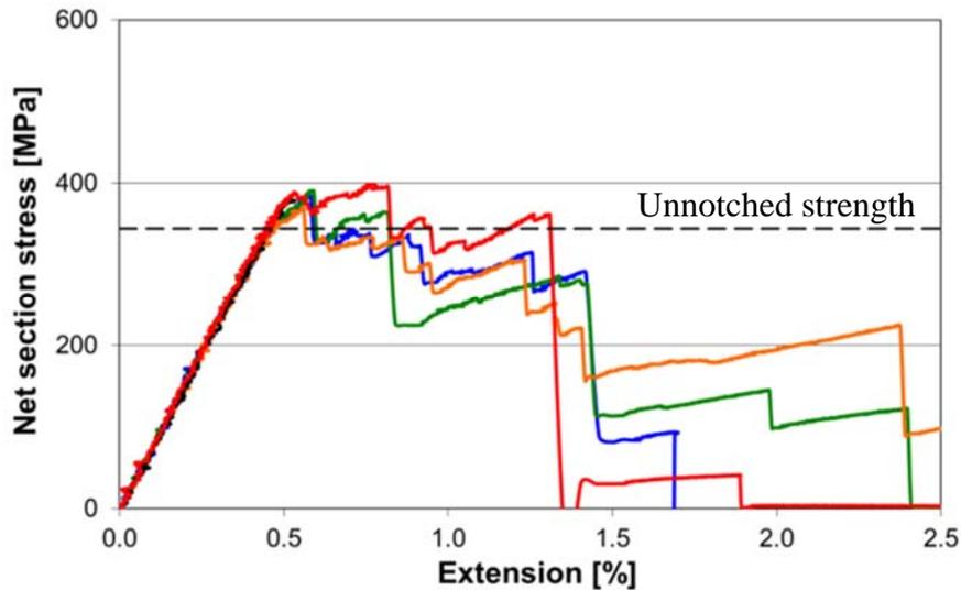
Figure 5. Open-hole tension of QI hybrid carbon specimens
