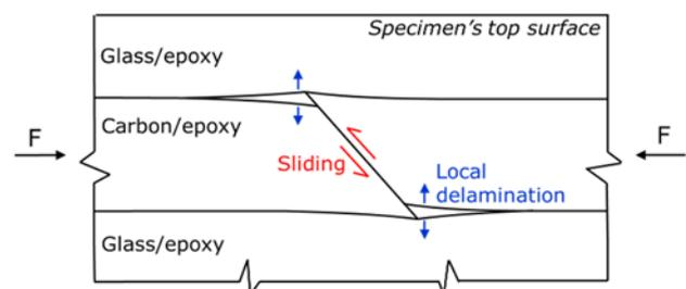
b) Side view schematic of micro-deformations
