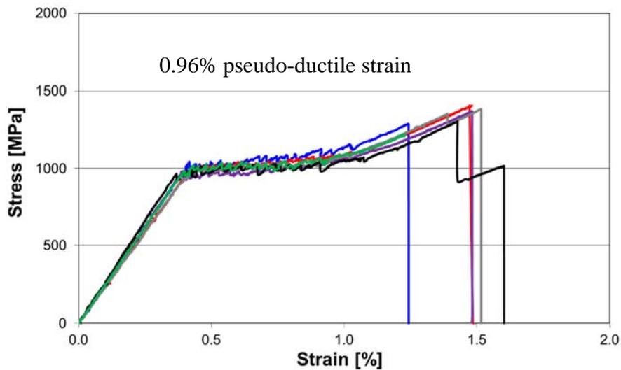
**Figure 3.** Stress-strain response for [T1000<sub>2</sub>/XN80<sub>2</sub>/T1000<sub>2</sub>] carbon hybrid [7]
