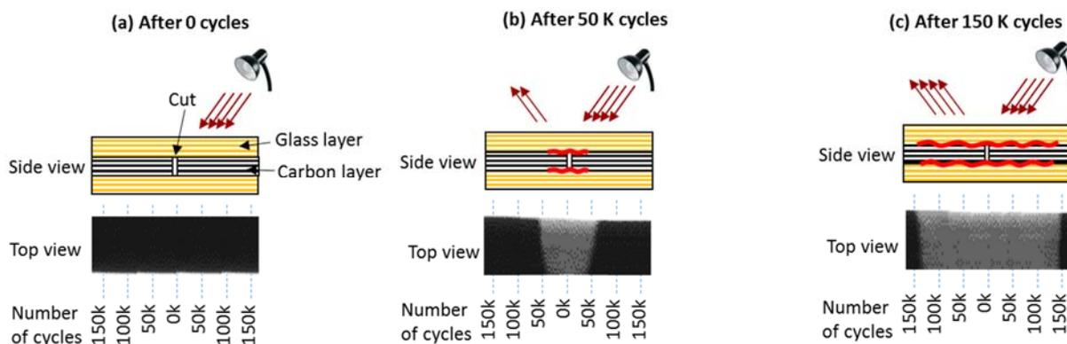
**Figure 8.** Fatigue sensor
