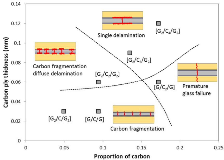
**Figure 2.** Damage mode map for E-glass/thin carbon hybrid composite [3]
