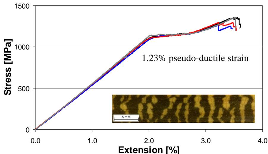
**Figure 1.** Pseudo-ductile response of S-glass/high strength carbon hybrid [2]
