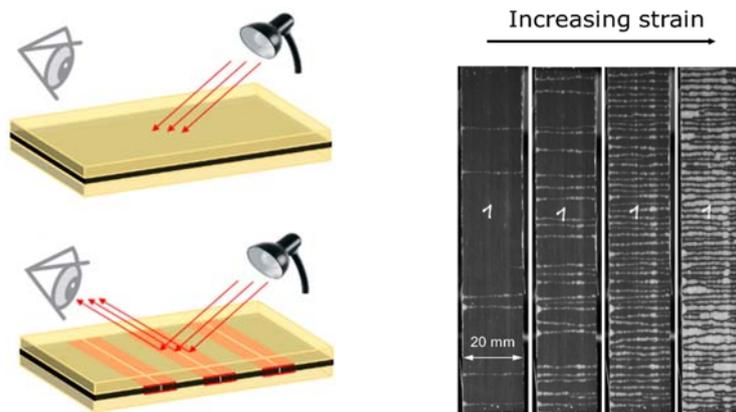
**Figure 7.** Visualisation of overstrain in glass-carbon hybrid
