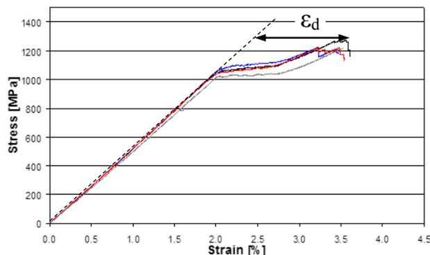
**Fig. 2 Pseudo-ductile strain  $\epsilon_d$  in glass/carbon thin ply hybrid**
